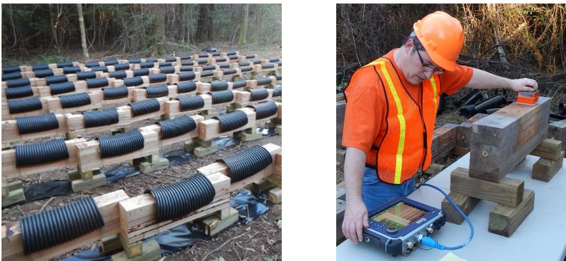
Figure 5. Specimens as positioned on site, and GPR scanning of specimens.
