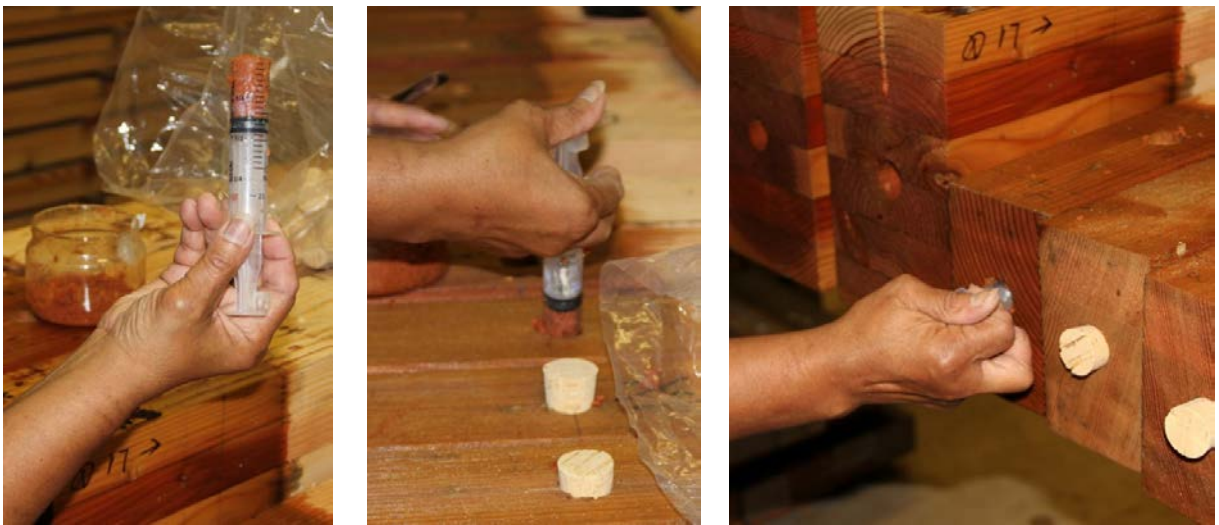
Figure 4. Inoculating specimens with Fomitopsis pinicola , brown-rot.
