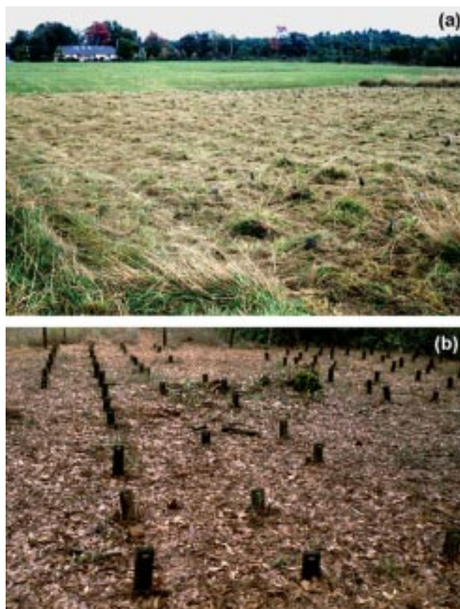
Figure 2—Ground-contact field trials: (a) exposure site; (b) test stakes.
