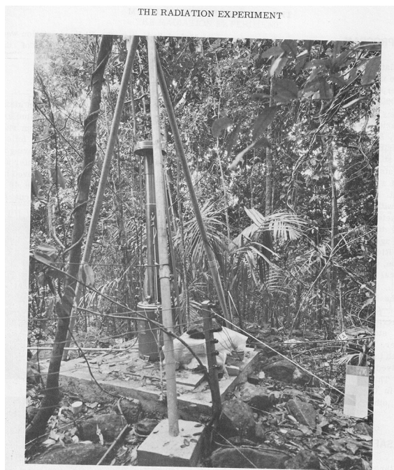
Fig. 4 Picture of the radiation source installed in a wet forest at El Verde, Luquillo Experimental Forest. The two-Mg lead container at the center of the concrete base contains the radioactive Cs source, which would be magnetically hoisted to below the oval metal structure when in operation (from Odum and Drewry 1970)
