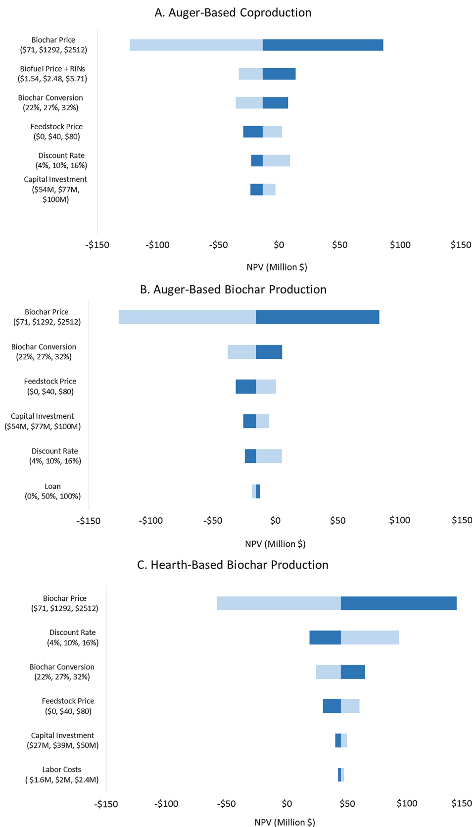
Fig. 5. Sensitivity tornados that illustrate the sensitivity of NPV to the random variables in the analysis. Dark shaded bars indicate an increase in value of the input variable and light shaded bars indicate a decrease in input variable value over the base case value.
