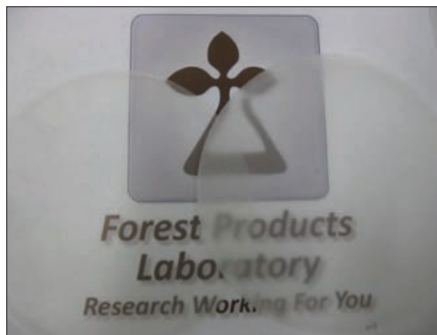
3. Visual images of CNF films made of CNF-0.5 h (right) and CNF-11 h (left). Diameter and thickness of the films were approximately 15 cm and 30 \mu m, respectively.
