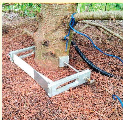
An electronic dendrometer fitted around a tree stem. The sensor recorded the stem’s diameter every 30 minutes, enabling researchers to determine when annual diameter growth stopped.
