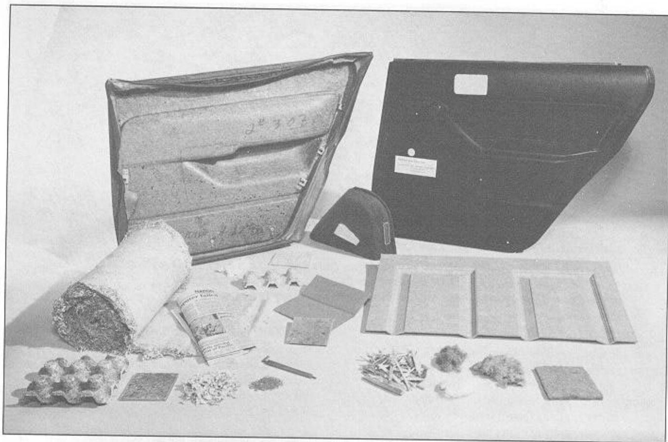
Figure 13—Composites that combine recycled wood fiber and plastic show great potential for a variety of uses, such as car door liners, decorative moldings, and other molded or sheet products.
