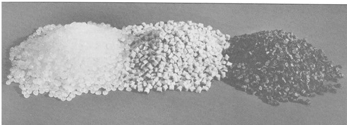
Figure 12—Putting recovered fiber into a form that manufacturers can readily use is a key step in recycling. FPL researchers have found a way to recombine plastic pellets (left) with wood fiber (center) or old newspapers (right) into a wood-plastic pellet that is readily used in existing plastics equipment.
