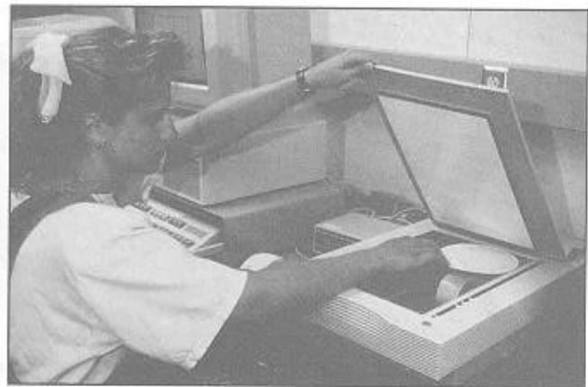
Figure 8—Contaminants are a major problem for papermakers using recycled fiber. Technology developed at the Forest Products Laboratory can easily and quickly measure the level of adhesive contaminants left in a recycled pulp.
