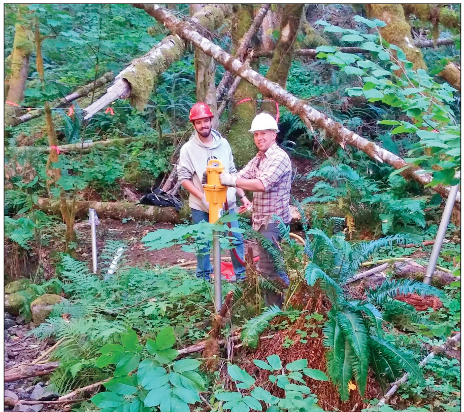
Graduate students Rob Pennington (left) and Jason Brandes install new wells that tap into the hyporheic zone of a stream in the H.J. Andrews Experimental Forest.
