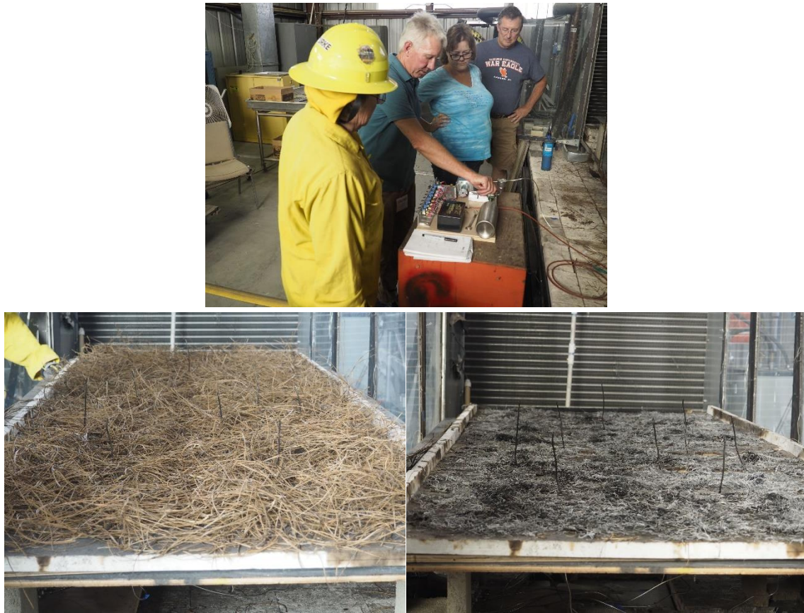
Figure 4 - Canister gas-sampling system with manifold (top) used to sample pyrolysis and flaming combustion gases from longleaf pine needle fuel beds through stainless steel tubes (bottom).
