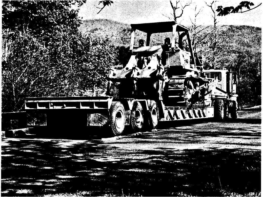
Figure 1.—Loaded rear-axle trailer used for load testing the Press-Lam bridge. (M85 0023- 17)
