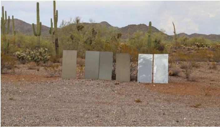
Figure 17.—Sample galvanized steel and powder coated panels. Photo by Brandon Colvin, U.S. Bureau of Land Management.
