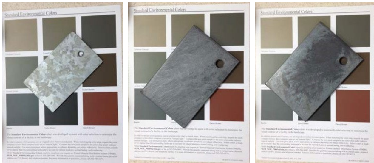
Figure 6.—Valmont galvanized steel samples overlaid onto BLM standard color chart. Photo by Brandon Colvin, U.S. Bureau of Land Management.
