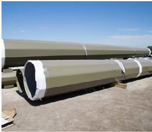
Figure 19.—Monopole production at Valmont manufacturing: a) welding; b) steel work complete; c) ready for powder coat; d) ready for transport. Photos by Brandon Colvin, U.S. Bureau of Land Management.
