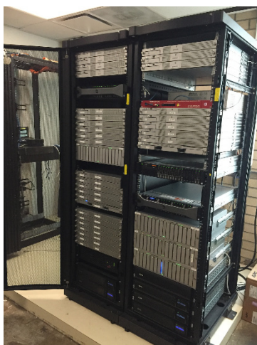
Figure 2: The FireBuster forecast model runs on a 40-core Dell PowerEdge R820 server. Mass storage systems are used for archived data. Another server (not shown) converts model output to web-displayable graphics.
