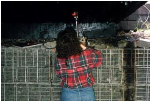
Figure 8—Electrical resistance moisture meter used for measurements.
