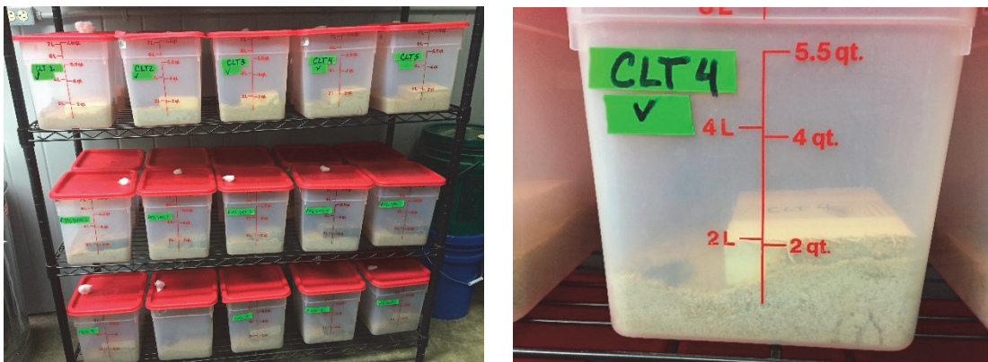
Figure 2. Test containers for Reticulitermes sp. lab scale test (left) and mud tube construction on the vertical face of CLT test block (right).
