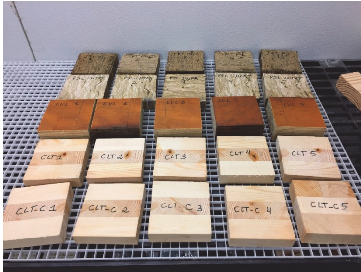
Figure 1. Conditioning test blocks to 12% EMC in an environmental chamber.
