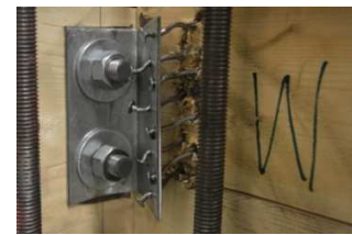
Fig. 3- Wall-to-floor angle bracket shear test
