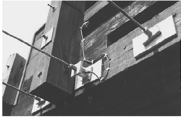
Figure 13—One of six load cells installed on stressing bars to measure changes in bar force.
