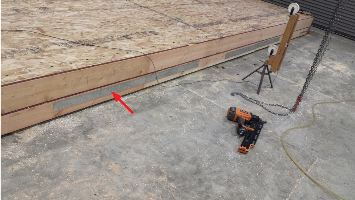
Figure 8. Chord strap from Simpson Strong-Tie CMSTC16 coil straps cut to 6-ft lengths for use in Part B SIP diaphragm tests.
