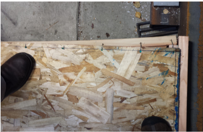
Figure 14. A typical failure mode at boundary framing of Part A diaphragms.
