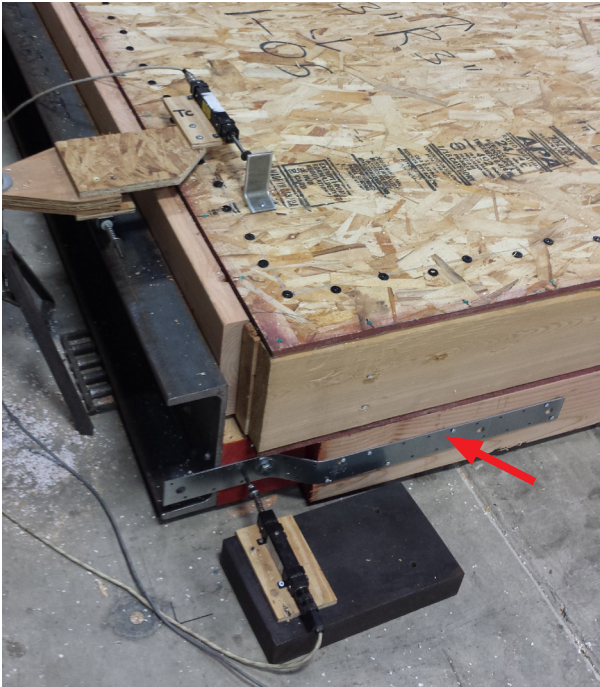
Figure 9. Framing anchor (Simpson Strong-Tie MSTI26) used in Part B SIP diaphragm tests.
