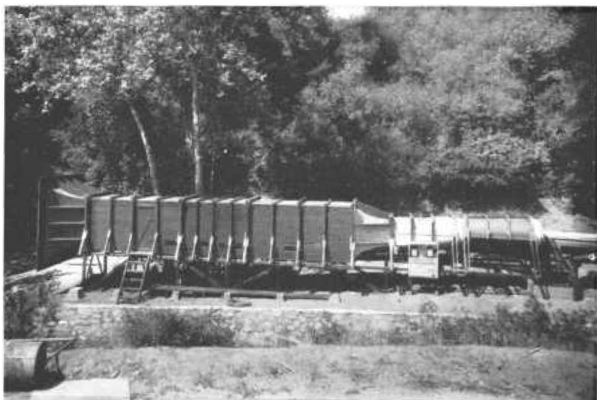
FIGURE 3.—Wind tunnel used in fire-behavior studies; test section is 30 feet long with a cross section 6 x 6 feet, over-all length 55 feet.
