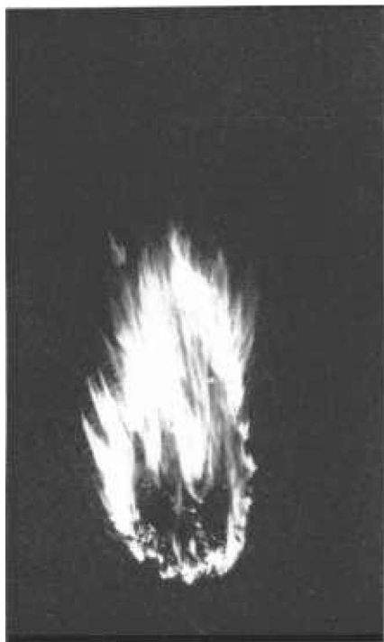
FIGURE 5.—Pine-needle fire 30 seconds after ignition, photographed from above; wind velocity 8 m. p. h.
