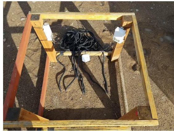
Figure 2. Control frame with soil moisture & temperature probes and RH sensor.
