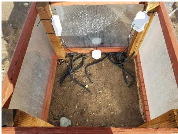
Figure 3. Clear frame with soil moisture & temperature probes and RH sensor. All four sides of the frame are made of corrugated Plexiglas
