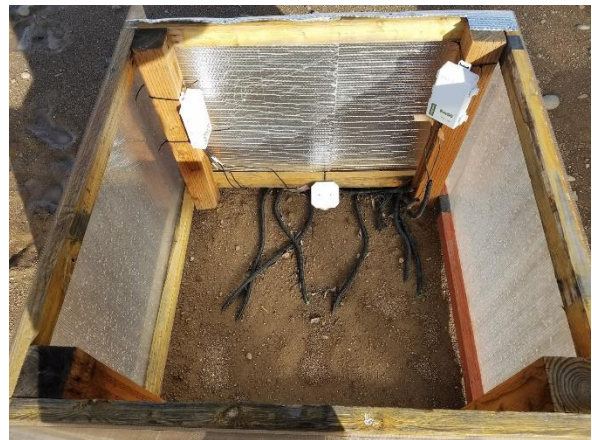
Figure 4. Solar frame with soil moisture & temperature probes and RH sensor. The east, south, and west sides of the solar frame are made of corrugated Plexiglas while the north panel is a reflective material.
