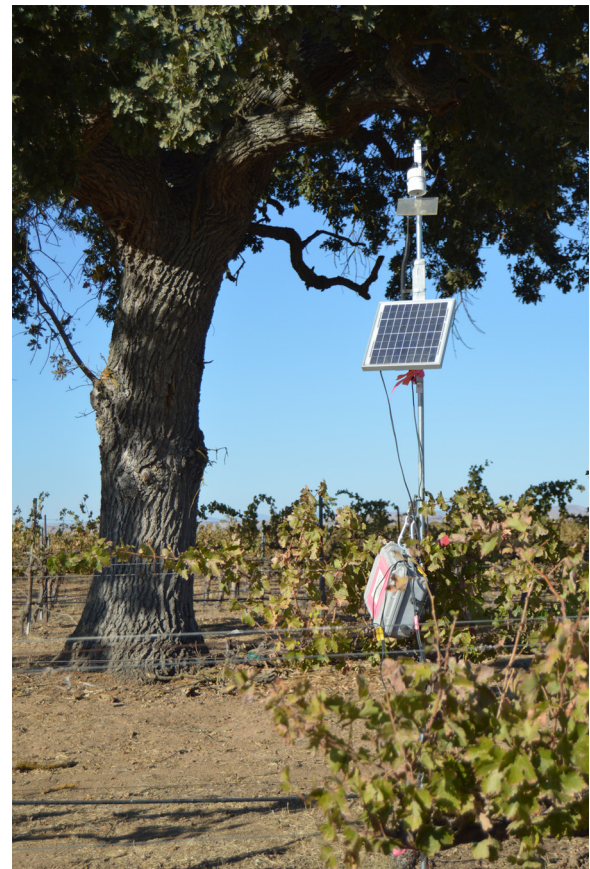
Fig. 2. Echolocation recording device at a tree site. The Anabat II detector echolocation microphone with a polycarbonate sound reflector plate is mounted at the top of a 3m metal post. The detector and battery (charged by a 10 W solar panel) are contained within a weather-proof container that is connected to and hangs from the post. (Photo by S. Giordano).
