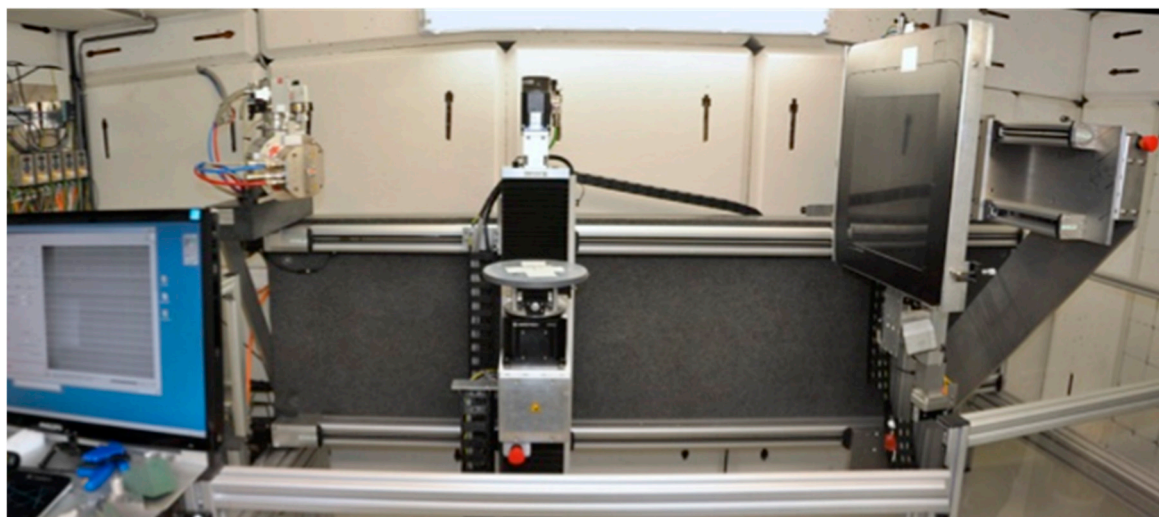
Figure 17. A micro-computed tomography ( \mu CT) system in use at Ghent University [285].
