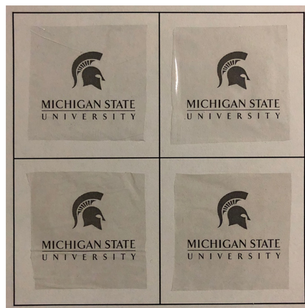
Fig. 5. Visual clarity of neat PLA (top left) and PLA/CNC nanocomposites films with 0.5% CNC (top right); 1% CNC (bottom left) and 2% CNC (bottom right).
