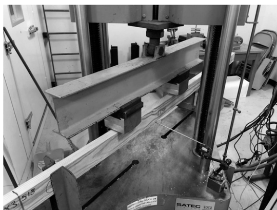
Figure 1. Static bending test setup as per ASTM D198-15.
