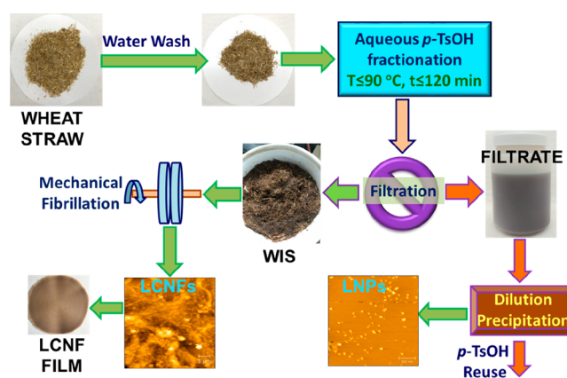
Figure 1. A schematic flow diagram showing fractionation of wheat straw and productions of LCNFs and LNPs.
