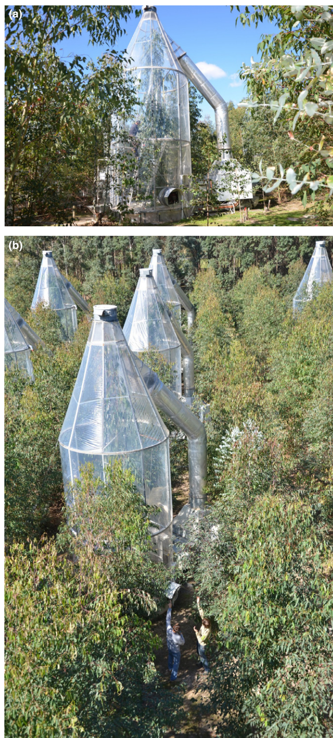
Fig. 1 Whole-tree chambers near Hawkesbury, New South Wales, Australia. (a) Closer view of a chamber and the air-handling and control equipment. (b) Chambers used in the Drake et al. (2019a,b) experiments in the context of the surrounding plantation. Photographs © Sebastian Pfautsch, used with permission.
