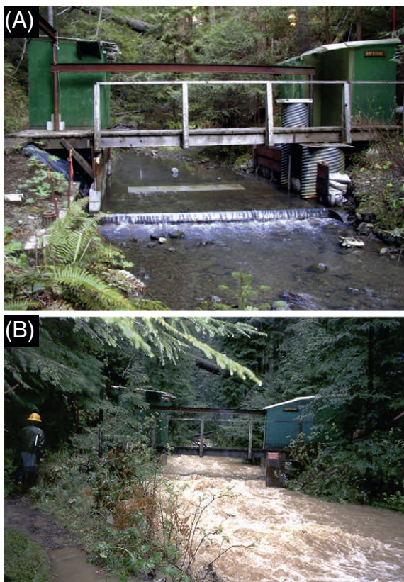
Fig. 3. View of the study reach in North Fork Caspar Creek showing the Arfstein gauge and bedload traps site during low (A) and high flows (B).
