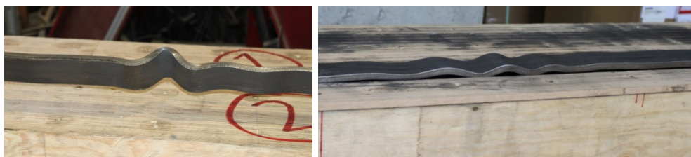
Figure 14: Failure mode of Specimen 3 (left) and Specimen 4 (right).
