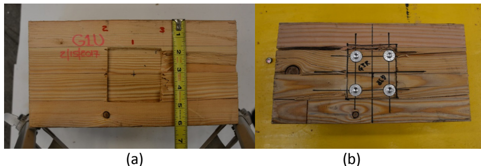
Figure 2. Glulam specimens post-test: (a) no screw reinforcement; (b) 2 in. x 2 in. reinforcement.
