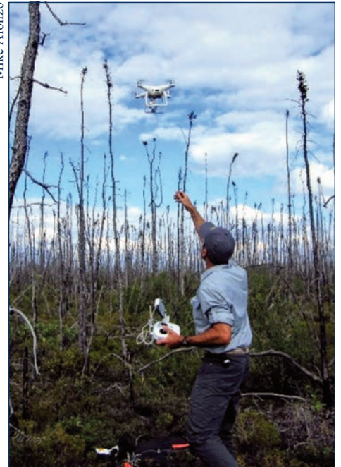
A researcher catches a drone outfitted with a camera. The resulting images were converted to a 3-D point cloud from which the researchers could calculate tree density, species composition, and above-ground biomass with a high degree of accuracy.
