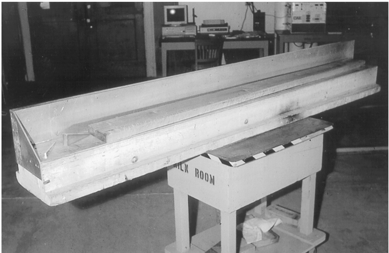
Figure 1—Warp measuring table and wedges used for measuring twist.
