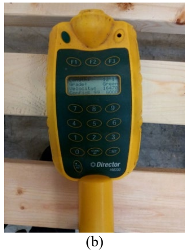
Figure 4 —Longitudinal vibration test setup used in this study: (a) test setup; (b) fibre-gen model HM 200 Hitman equipment used to conduct longitudinal vibration tests.
