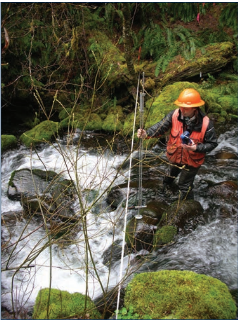
A researcher measures the amount of water and rate at which it moves. Stream discharge measurements allow scientists to model streamflow to better understand seasonal habitats. Streamflow is a driver of habitat connectivity and of the shifts in habitat functionality throughout the year.
