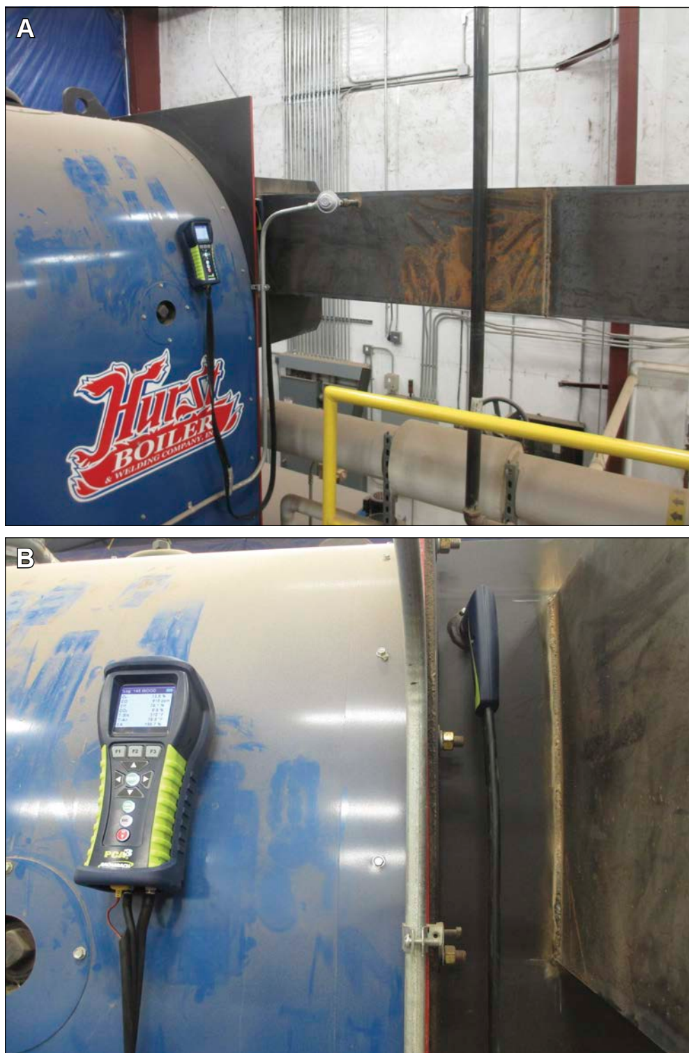
Figure 1—(A) Wood energy burner at Delta Junction High School; (B) closeup of combustion gas analyzer showing insertion point for sampling.
