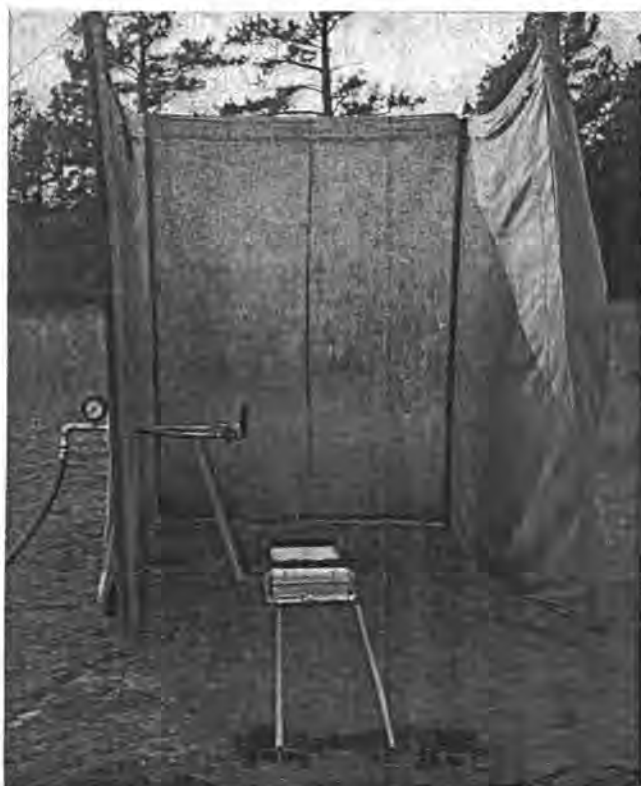
Figure 4.—Rocky Mountain infiltrometer used to apply rain to small plots to obtain rates of water absorption, runoff, and erosion under different conditions of vegetation, soil, and use. (Manitou Experimental Forest)
