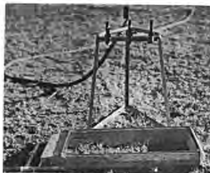
FIG. 1 Rocky Mountain infiltrometer installed on a grassland site at Manitou Experimental Forest. Rainfall simulator equipped with three type F nozzles. Rain troughs are located on both sides of the 2.5 sq ft plot.
