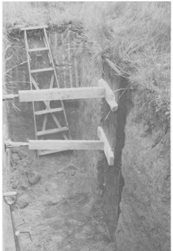
FIG. 2. Nail-board being inserted into trench wall for root-sample excavation.
