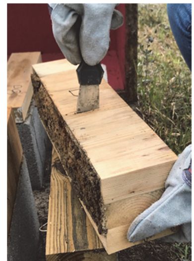
Figure 6. Field testing of CLT sections in AWP E21-18 setups. Left - initial setup of test pieces and controls on concrete blocks with internal feeder stakes; Middle - 24 months of exposure, exhibiting shelter tube formation between concrete support block and CLT test block; Right - hollowed CLT test block, with apparently sound exterior, after 24 months of exposure.
