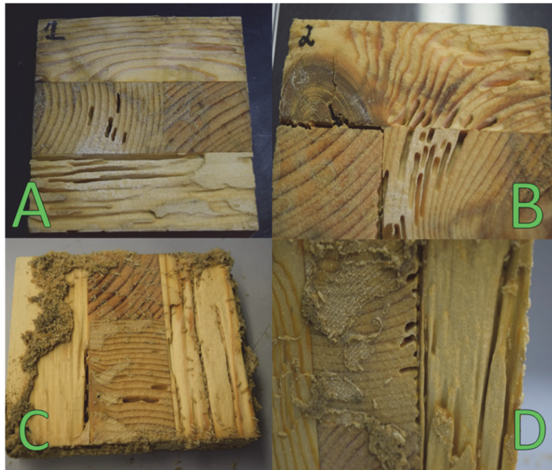
Figure 3. Revised test blocks of smaller thickness (1-inch) following exposure to Reticulitermes sp. Excavations can be seen on the exposed surfaces of blocks A and B post-cleaning. Blocks C and D show active termites immediately after removal from test containers, with intact shelter tubes.
