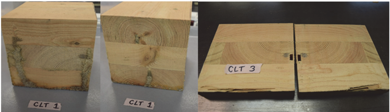
Figure 2. 4-inch cubes after eight weeks of testing. Left – immediately after testing, with mud tubes intact; Right – test block sliced open to determine depth and location of termite tunneling.
