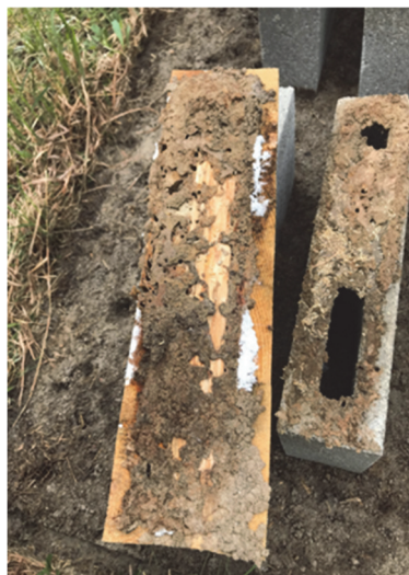
Figure 6. Field testing of CLT sections in AWP E21-18 setups. Left - initial setup of test pieces and controls on concrete blocks with internal feeder stakes; Middle - 24 months of exposure, exhibiting shelter tube formation between concrete support block and CLT test block; Right - hollowed CLT test block, with apparently sound exterior, after 24 months of exposure.
