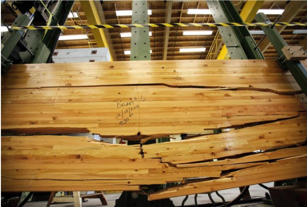
Figure 1. Failure of one of twelve 72-foot glulam beams that failed under loads between 69,000 and 95,800 pounds after up to a 13 inch deflection (Posted on January 28, 2013 by James T. Spartz https://www.fpl.fs.fed.us/labnotes/?p=72 ).
