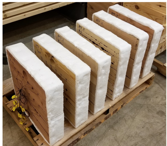
FIGURE 1 Six wood specimens wrapped in ceramic fiber batting [Colour figure can be viewed at wileyonlinelibrary.com ]
