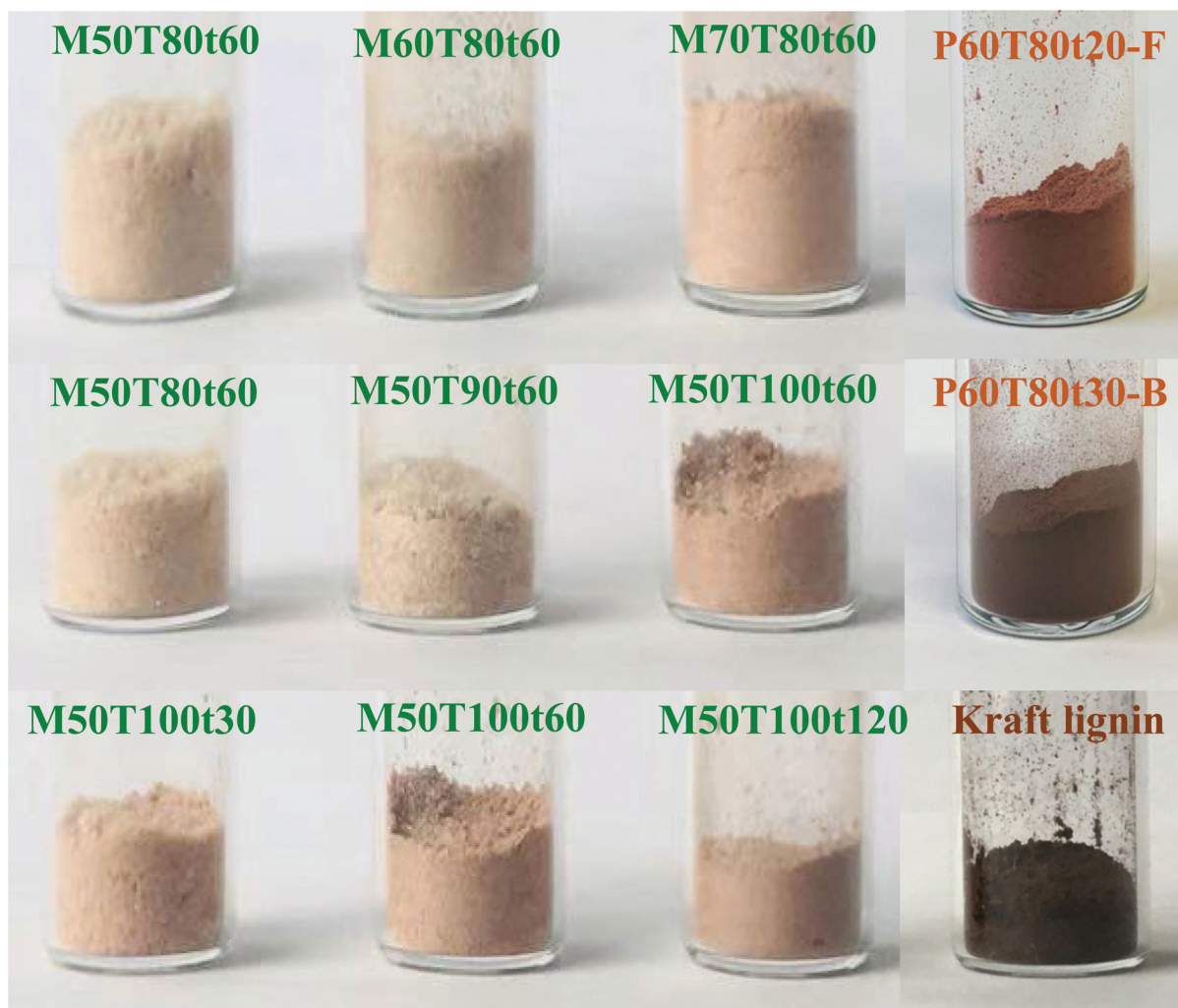
Fig. 6 Images show the color of dissolved wood lignin from MAHF under various conditions in comparison with lignin from AHF using p -TsOH and kraft pulping.
