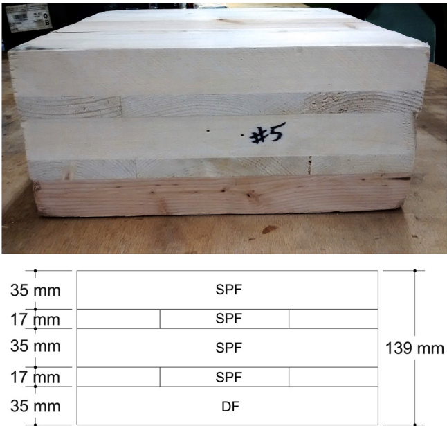
Fig. 1. One of the CLT samples used for making small-scale specimens (top); schematic cross-section (bottom).
