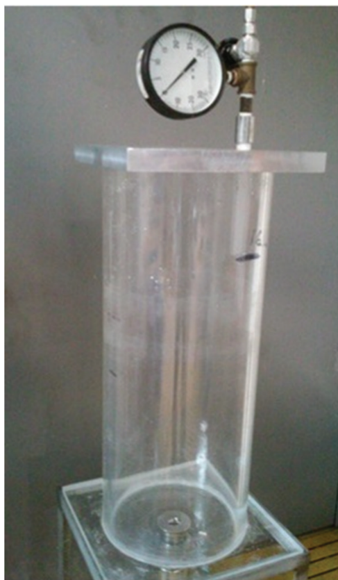
1. Batch bench-scale unit (left); the black mark indicates 16 L volume. Schematic of the two continuous processes (right).
