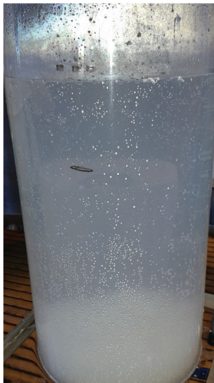
3. Surface of the liquid after the vacuum has been released (left). Tube at the end of the experiment showing the settled fiber (right).
