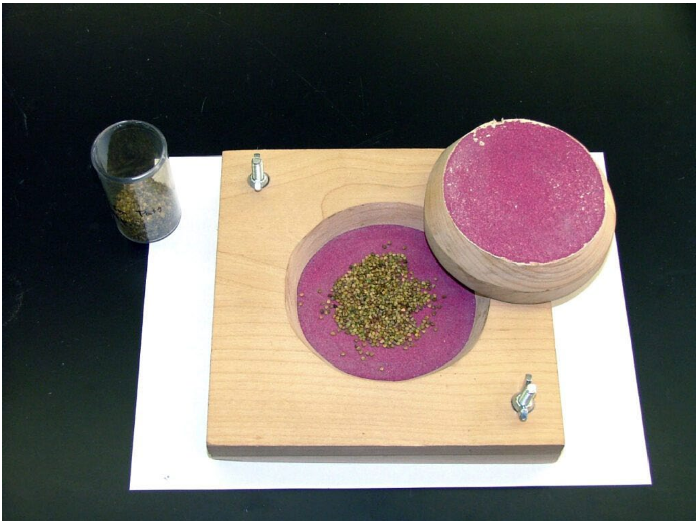
Figure 9. Apparatus used to mechanically scarify prairie clover seed with sand paper. Photo: S. Bushman, ARS.
