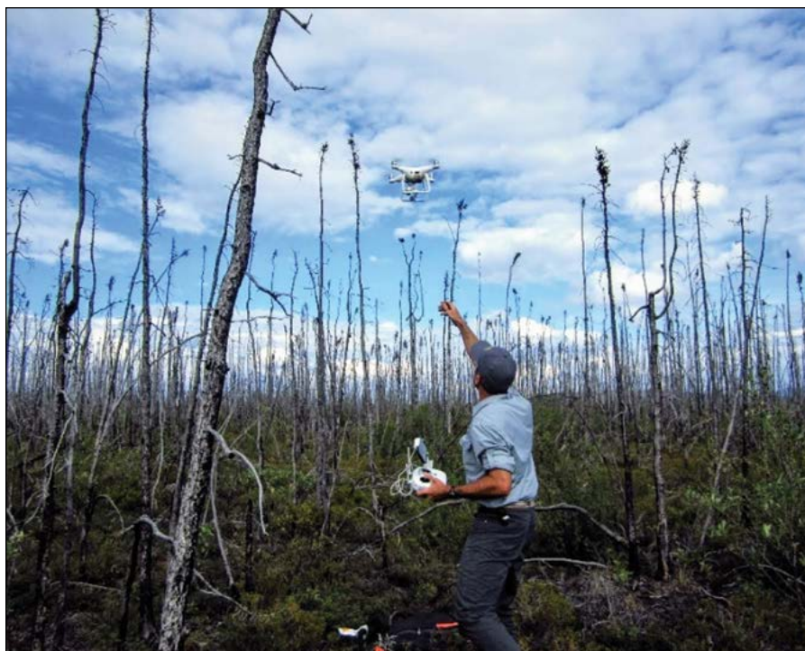
A researcher catches a drone outfitted with a camera. The resulting images were converted to a 3-D point cloud from which tree density, species composition, and aboveground biomass are calculated with a high degree of accuracy.
