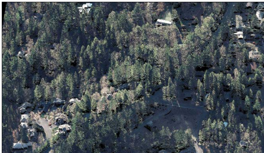
A perspective 3D view generated by the fusion of LiDAR data and high-resolution aerial photographs enables precise measurements of tree height and other objects.
