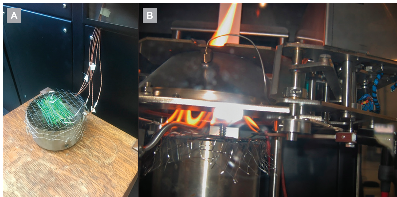
Figure 1 —(A) New cone calorimeter holder with longleaf pine needles bedding constrained between wire grids, and (B) test specimen flaming as it is exposed to 35 \text{ kW m}^{-2} in the cone calorimeter.
