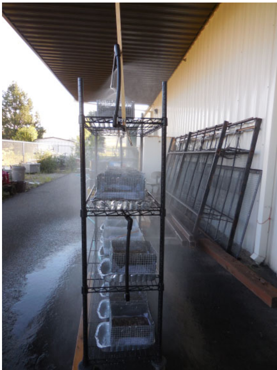
Fig. 4. An entire set of 39 fuelbeds was placed under a set of water sprinklers for 25 h to bring the woody fuels to saturation. Sprinklers were placed at each level.
