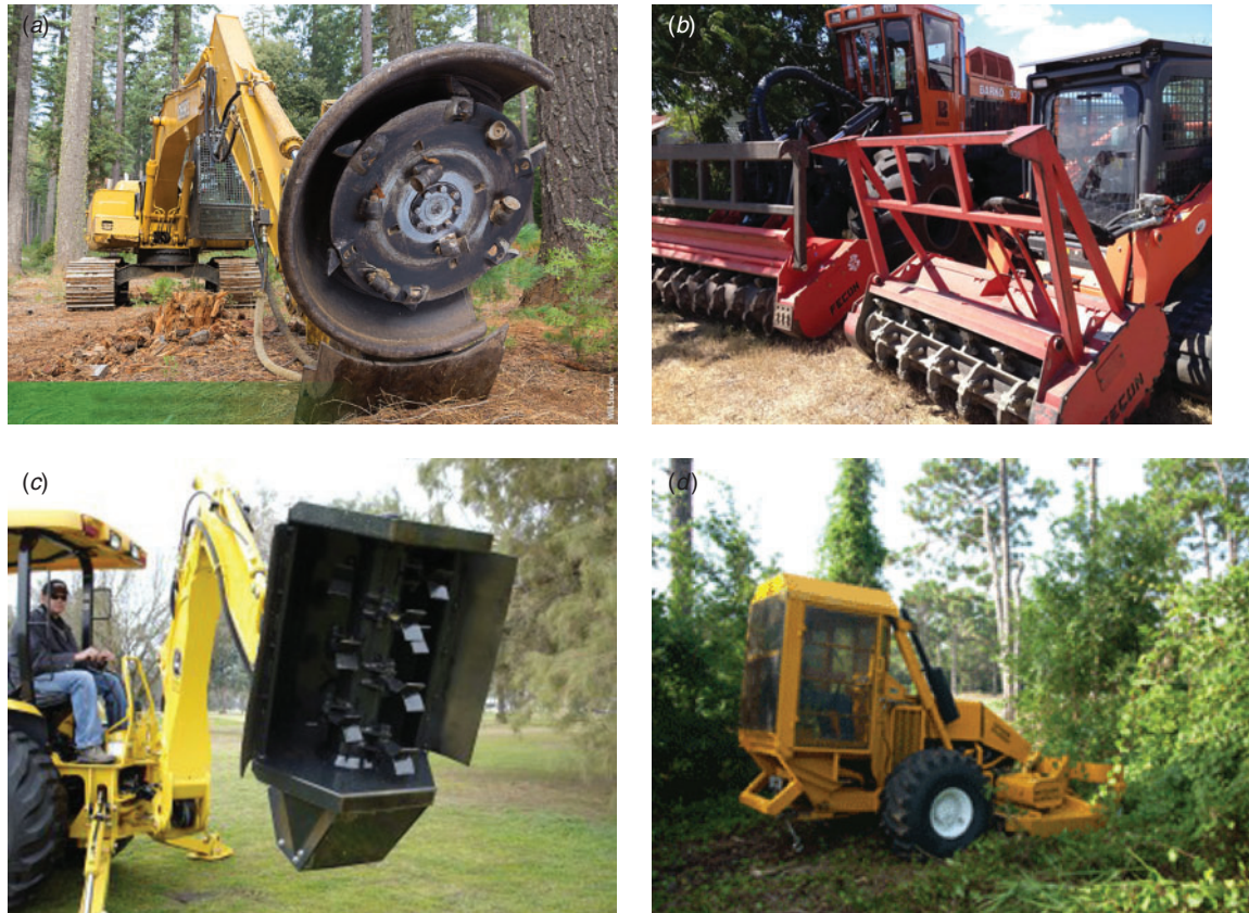
Fig. 1. There are two primary equipment types most commonly used for mastication (also referred to as mulching) treatments. Cutting tools placed on either a (a) vertical shaft (VS) (photo from amacocei.com, accessed 9 October 2018), or (b) horizontal shaft (HS) (photo from txbrushcutter.com, accessed 9 October 2018) using different configurations, such as (c) fixed teeth, swinging hammers (photo from rockhound.com, accessed 9 October 2018), and (d) Kut Kwick bushmaster fire mower (photo from forestfireequipment.com, accessed 9 October 2018).
