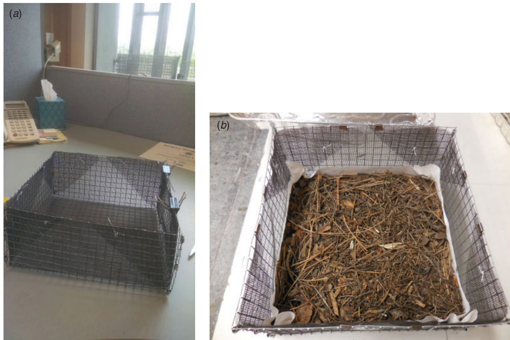
Fig. 3. (a) The synthetic wire cage used to build the masticated fuelbed using loadings for each of the 13 study sites; and (b) a recreated fuelbed for LG site (Table 1).
