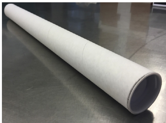
Figure 2 Cardboard tube (4 cm diameter, 42 cm long) used as a negative control to compare Pityophthorus juglandis landing rate on a host, Juglans californica (3.8 cm mean diameter, 40.7 cm mean length, n = 10 ) vs. a non-host without volatiles. Photograph by ID Lona. [Colour figure can be viewed at wileyonlinelibrary.com ].
