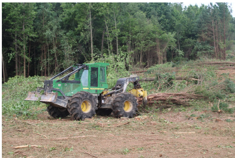
Figure 2. A grapple skidder pulling a load of pine trees (including branches and tops). Image credit: Dr. Patrick Hiesl, Clemson University.
