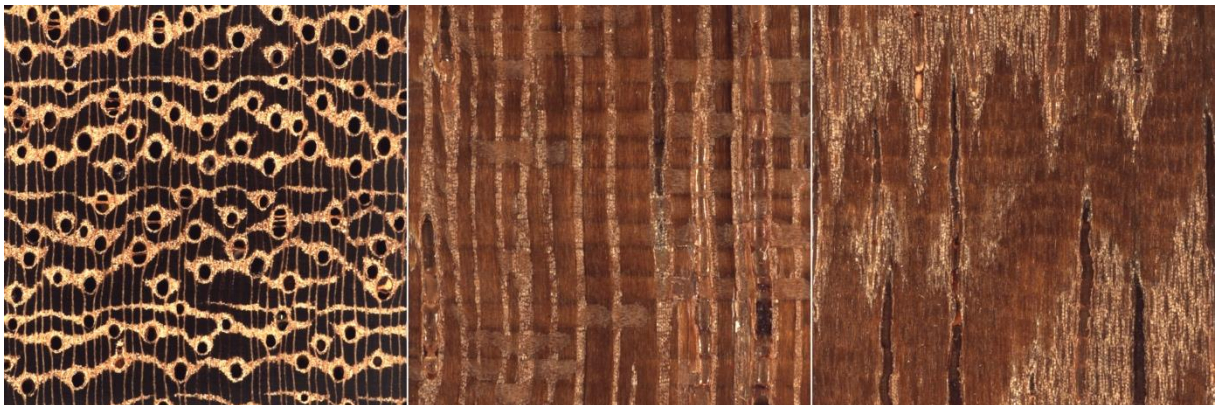
Fig. 3: XyloTron macrographs of Martiodendron sp. Transverse (left), radial (centre), and tangential (right) surfaces. Each image is 6,35mm x 6,35mm. Images courtesy of Richard Soares, Center for Wood Anatomy Research, Forest Products Laboratory, USA.
