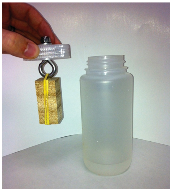
Figure 3. Sample setup for modified EN-717-3 method [44].
