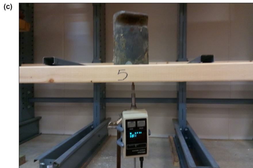
Figure 2. Flatwise bending test setup: (a) schematic diagram of test setup; (b) specimen being tested; (c) load being applied and corresponding deflection measurement.
